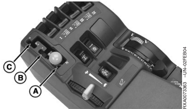
A—PARK B—Reverse Gears C—Forward Gears
