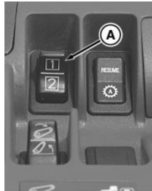
A—Sequence Switch B—Sequence Indicator C—IMS Indicator
