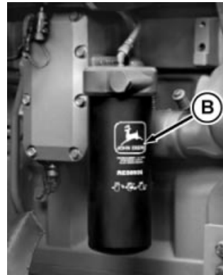
A—Drain Fitting B—Oil Filter
